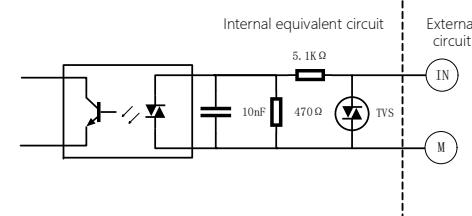
In the figure above, **M** is the common terminal of the external input signal, and **IN** is the external input signal.
