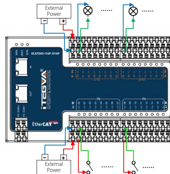
Note: The maximum drive current of the output signal is 500mA. Please check the external load rated power and internal resistance before use. If the load required current exceeds 500mA, increase the current limiting measure.
