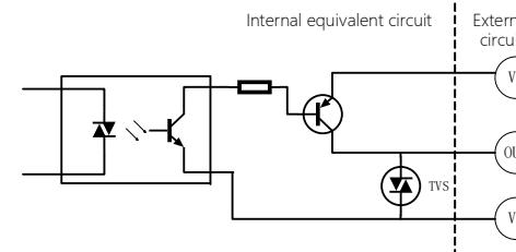
In the figure above, **V-** is the common terminal of external output signal and **OUT** is the output signal.
